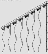
Vertical blinds system 2900, crank operated, max. length 6m
